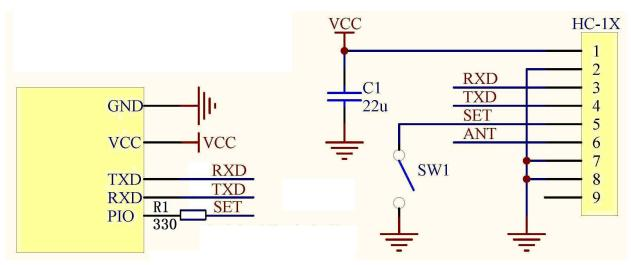
Please set the "SET" control pin to high level or hanging out in normal times, and set to low level in setting parameters state.
